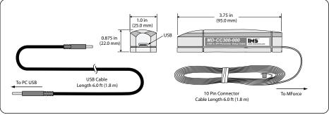
Figure A.2: MD-CC300-000 Mechanical Specifications
